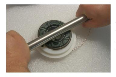
Press in the big spring with the help of a metal bar, keeping the bar in this specific position
