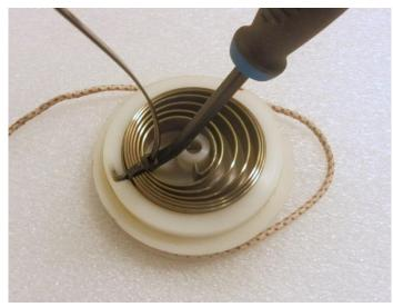
Remove the spring using as a lever a large and flat screwdriver
