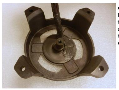
Grease the bottom of the flash starter and insert the thin plastic disk
