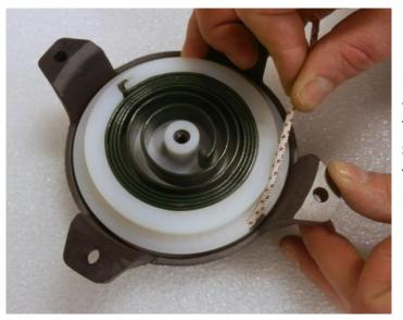
Insert the pulley paying attention to fix the small spring in the teeth of picture 2 of previous page
