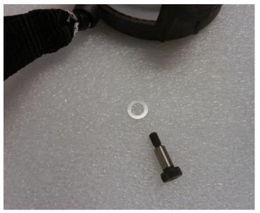
Take the tugger bolt and screw it on the pulley driver, using strong glue on the thread of the screw. Tighten the screw very firmly.
