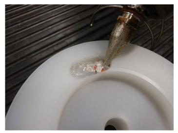
Fill the hole with hot glue and make sure the glue doesn't exit from the edge of the hole
