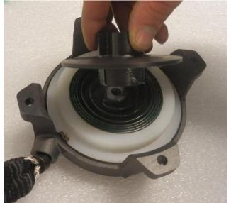
Place the pulley driver in its seat
