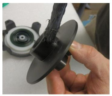
Grease the lower part of the pulley driver and the internal part of the big spring
