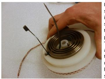
Lift up the spring to insert a safety clip in this specific position. This is to avoid that the spring unrolls and hits someone
